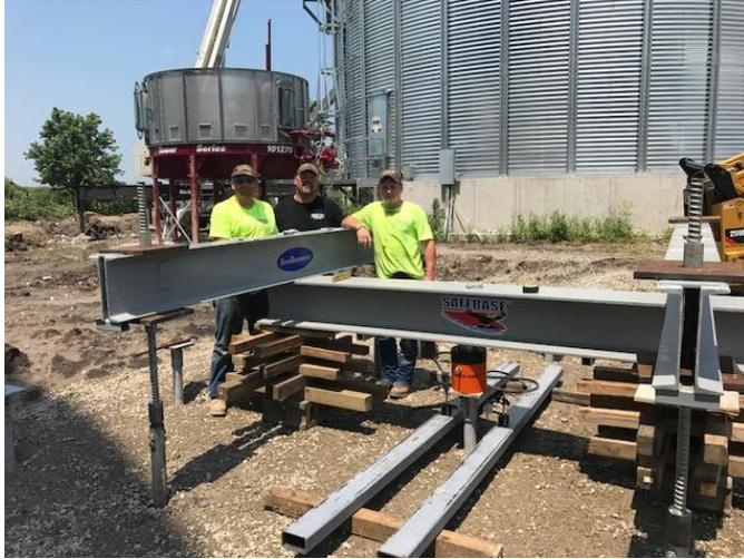
A compression test was performed to verify the capacity of the piers. A load of 96,600 lbs was applied to the pier and the total vertical displacement was .880" most of which was elastic shortening of the pile shaft. The plot of the test shows the blue line representing the load test on the pier staying near the red line representing the elastic shortening of the shaft.
